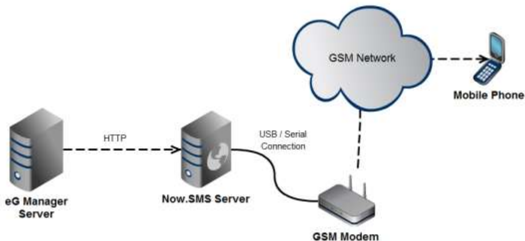
Figure 7.1: How the eG manager - NowSMS Lite integration works
