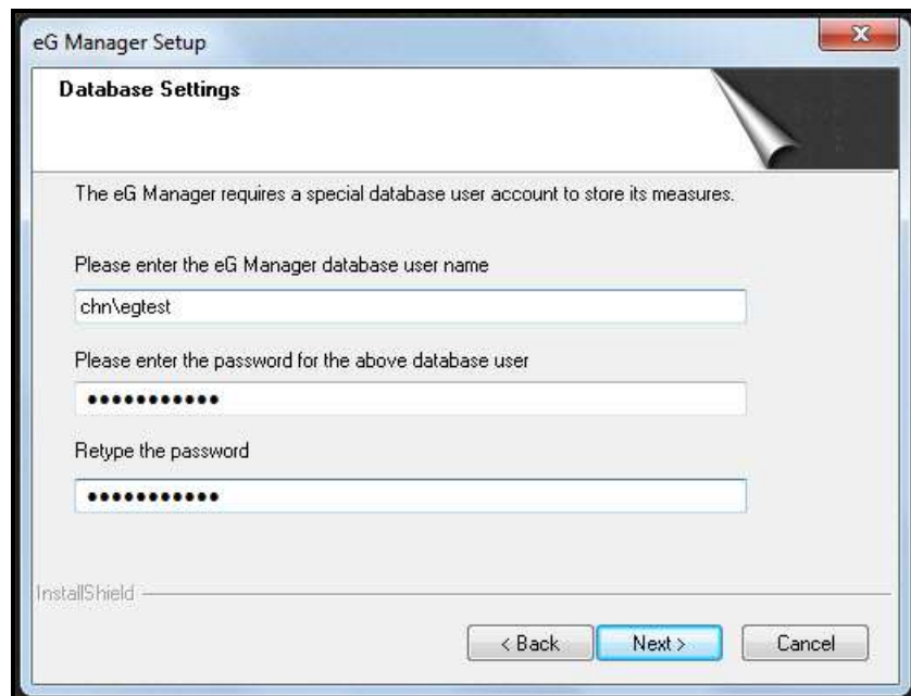
Figure 3.34: Specifying the user name and password to host the eG database on an MS SQL server with Windows Only Authentication enabled
