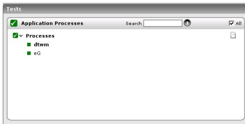
Figure 2.14: The Processes test that tracks the health of the Application Processes layer of a Linux server
