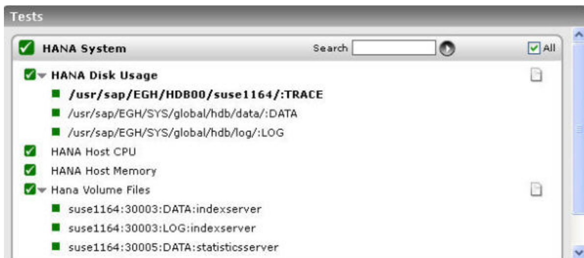
Figure 3.6: The tests mapped to the HANA System layer
