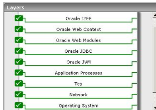
Figure 4.1: The layer model of the Oracle 10G application server
