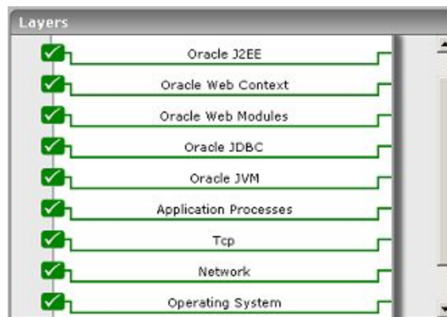
Figure 3.1: The layer model of the Oracle 9i AS
