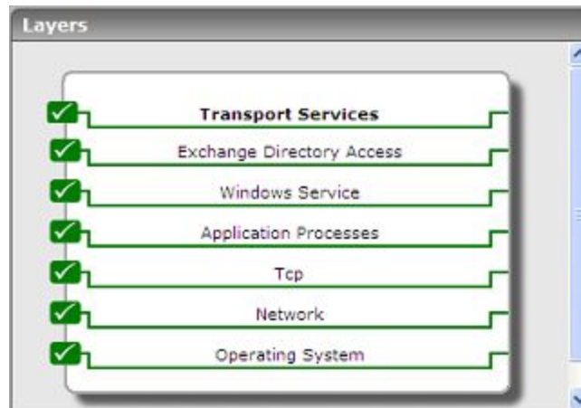
Figure 3.1: Layer model of the Microsoft Exchange Edge Transport server
