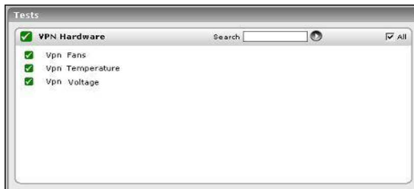
Figure 3.2: The tests mapped to the VPN Hardware layer
