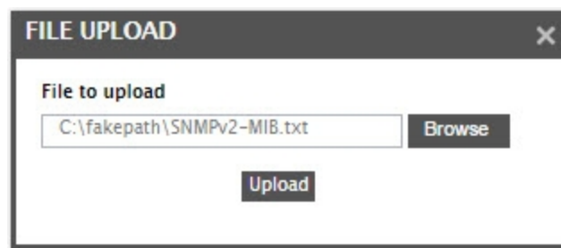
Figure 2.68: Specifying the full path to the MIB file to be uploaded
