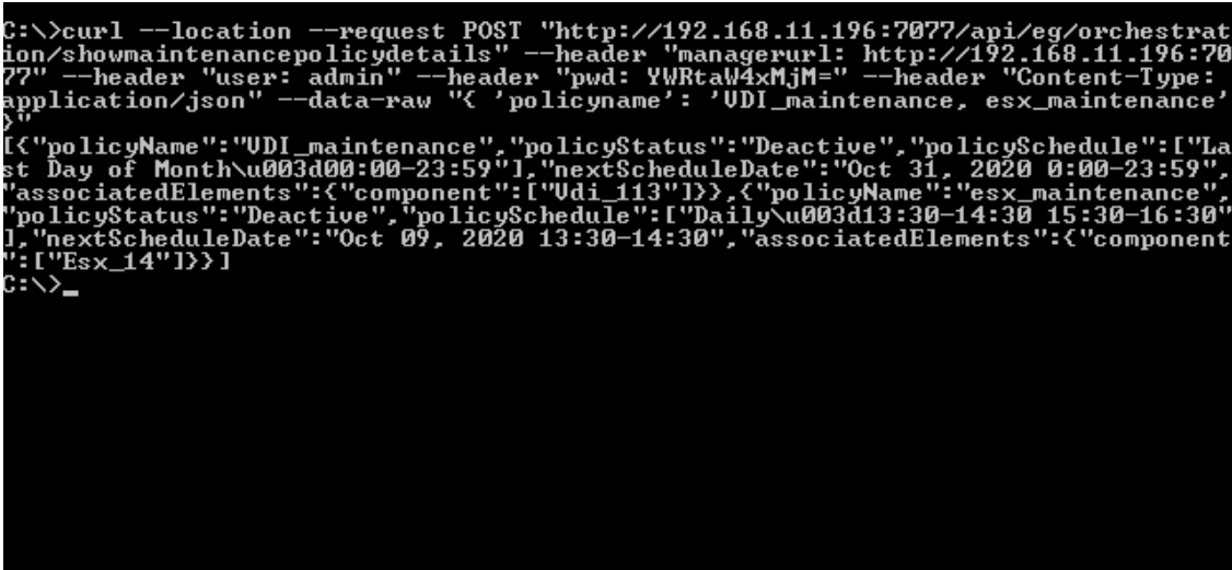
Figure 2.72: Displaying the details of the Maintenance Policies in the target environment using cURL
